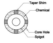
Step - 5: Once all the glasses are properly aligned pour chemical into hole
