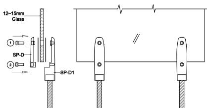
Step - 4: Install glass (with spigot) into core hole. Using Wooden blocks and shim, align spigots.
